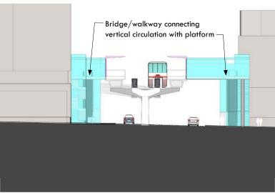
Figure 33: Cross Section
