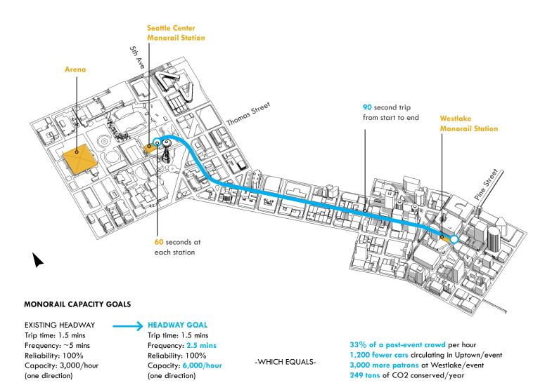
Figure 14: System Diagram
